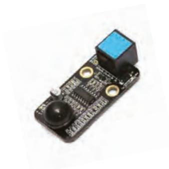
**Me 3-Axis Accelerometer and Gyro Sensor**
