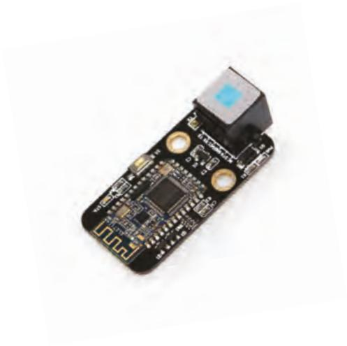
**Me Infrared Receiver Decode**
